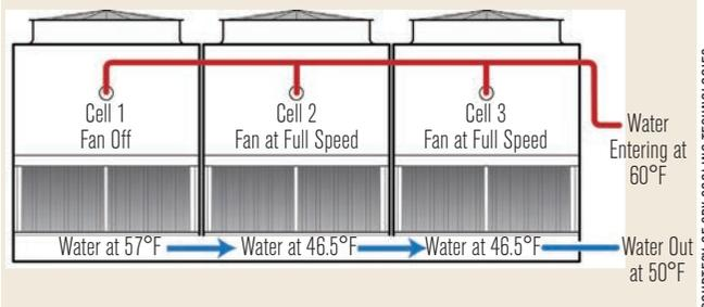
**FIGURE 5** Single cell with fan running has substantially lower leaving cold water temperature than the other two.
