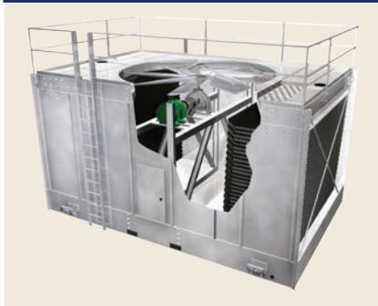
**FIGURE 7** Counterflow; water sprays downward, flows downward through the fill, and air flows in from sides and up through the fill. Water flow is counter to airflow.
