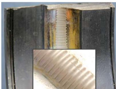
**FIGURE 2.** Fluting along a bearing race wall.
