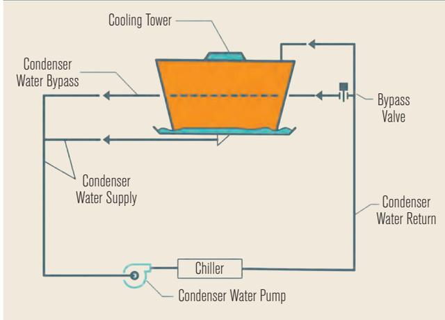
FIGURE 2 Correct cooling tower bypass.
