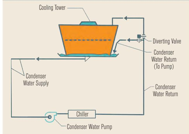
the tower. It is preferred to minimize the amount of horizontal pipe above the distribution basin. Where that cannot be avoided, an inverted water trap on the hot water pipe at the inlet to the distribution basin will limit the pull down volume. A functioning check valve on the condenser water pump will restrict water from falling back to the collection basin through the tower discharge pipe.
