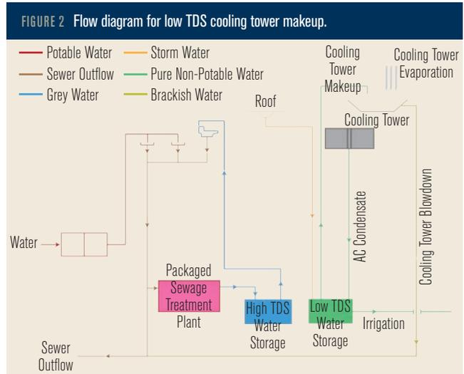
FIGURE 2 Flow diagram for low TDS cooling tower makeup.
