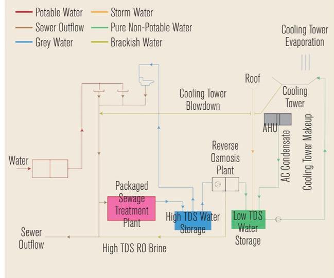
per gallon of product per day of capacity. The system portrayed in *Figure 3* is a portion of the treated sewage effluent for flushing, and the remainder of the effluent is subjected to RO treatment for either cooling tower makeup or irrigation.
