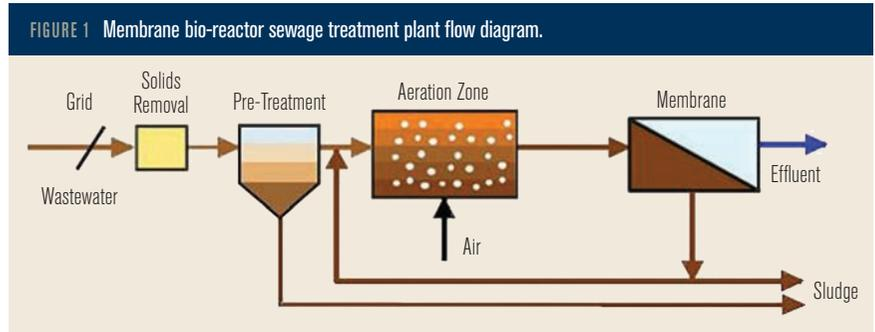
FIGURE 1 Membrane bio-reactor sewage treatment plant flow diagram.
